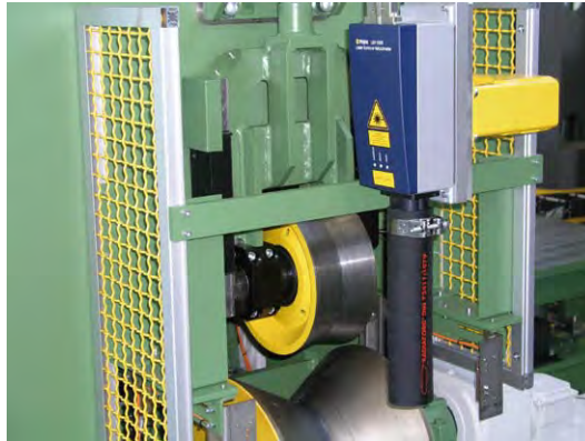
Fig. 5: The second Velocimeter follows the third driver.
