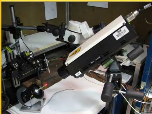
Fig. 3: Measuring the vibration stimuli using a laser vibrometer head with the laser focused on the mini shaker tip (lower image), in combination with the vibrometer controller (upper image).
