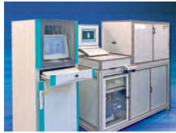
Figure 3: Station constructed for 100% quality control of nebulizer membranes.
