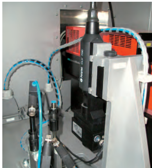
Figure 5: Integration of the Compact Laser Vibrometer equipped with a beam deflector on the test stand
