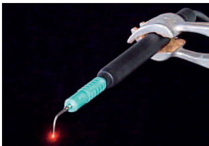
Figure 2. The laser from the Scanning Vibrometer is scanned over the surface of a dental ultrasonic scaler.
