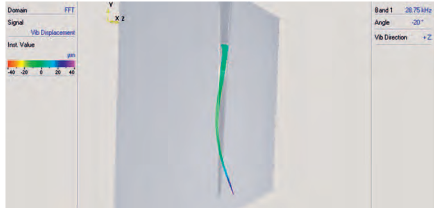
Figure 4. A snapshot from an animated deflection shape of the vibration data, superimposed over a video image of the scaler.
