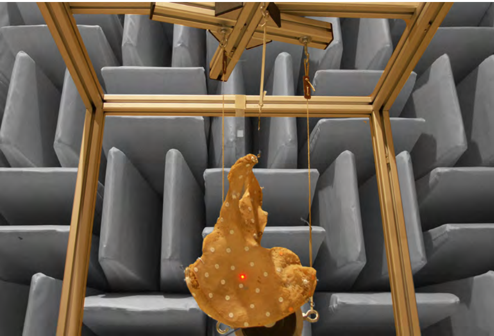
Figure 1: Suspension of the hip bone on rubber bands (red spot: focus point of the laser beam).
