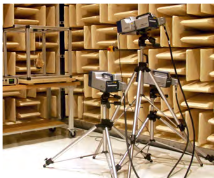
Figure 2: Test setup with a 3D scanning laser vibrometer.
