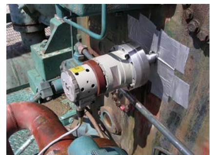
Figure 1: HBM Torsiograph with stub shaft mounted on oil pump, end of compressor (no longer manufactured).
