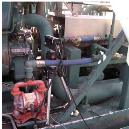
Figure 3: Rotational vibrometer mounted on a tripod.
