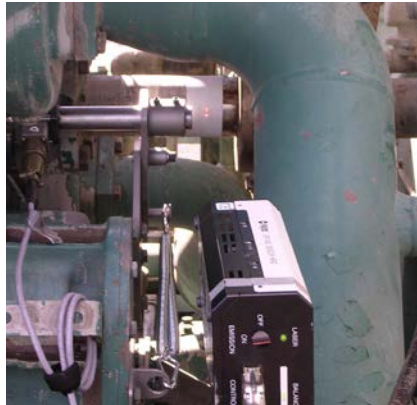
Figure 2: Laser rotational vibrometer aimed at reflective tape on shaft.
